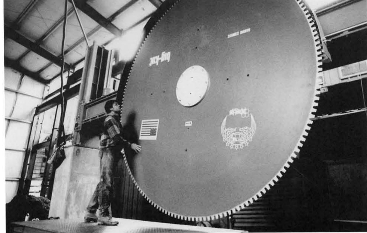
High-tech block saw being installed.
